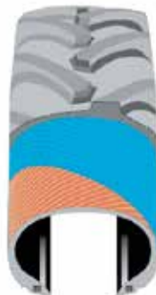
Bias tire construction: the cords are placed diagonally with certain degrees for the rotation direction of a tire.
